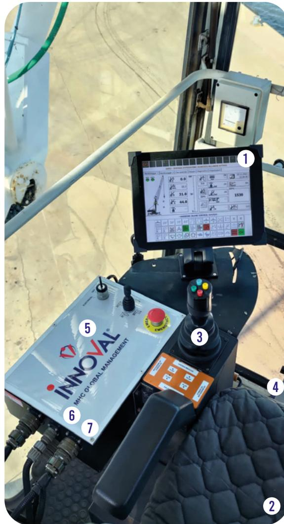
1. **Display** touch-screen VGA with integrated virtual keyboard
